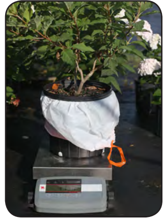
Figure 57. Weigh the nested container before and after irrigation
