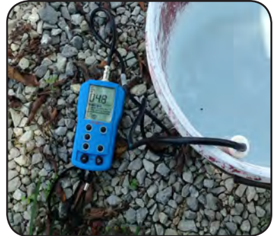
Figure 13. Use an EC meter to estimate water salinity
