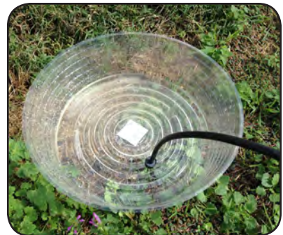
Figure 42. Place emitters directly into capture containers
