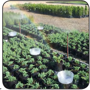
Figure 41. Set capture containers in a grid pattern above the canopy
