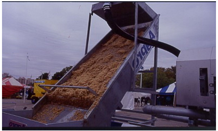
Figure 2. Static-screen separator. Source: Author Photo
