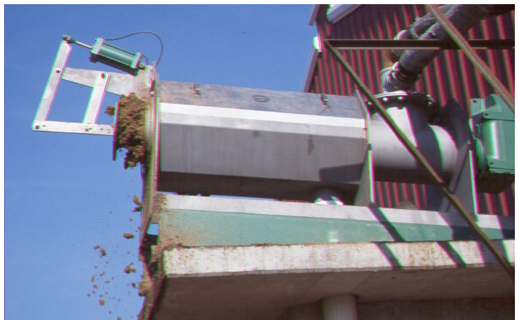
Figure 4. Screw-press separator. Source: Author Photo
