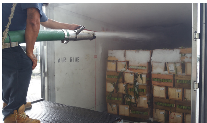
Figure 19. Flaked ice being blown on top of the cold crop as it is loaded into the refrigerated trailer. Photo: S.A. Sargent
