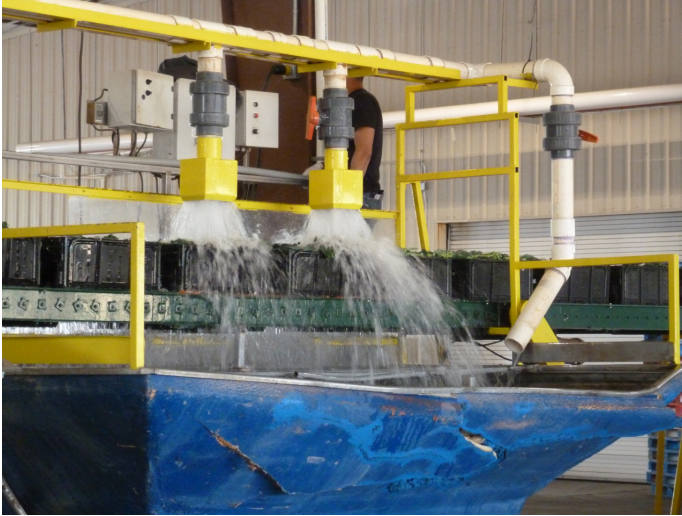
Figure 11. Slurry icing reusable plastic containers. The proportion of ice in the slurry can be varied depending on how much cooling and residual ice are needed. The cold water is sanitized and reused. Photo: T. Björkman
