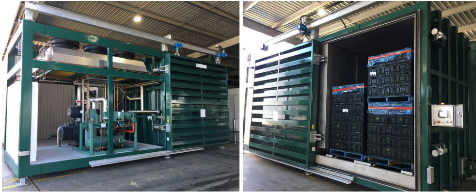
Figure 17. Vacuum chamber for four pallets. The vacuum pump and mechanicals are on the left, the chamber on the right. The whole unit can be shipped on a flatbed trailer. Used with permission of Quik-Cool Australia Pty Ltd.
