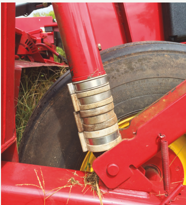
Figure 11.4. Mowers can be adjusted to cut native grasses at a proper height, about 8 inches, by several means. One of the easiest is to use cylinder stops as seen here. Credit, J. Walton.
