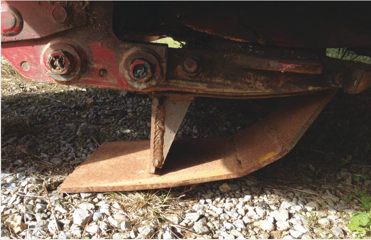
Figure 11.5. Skid shoes are another effective way to adjust mower height. Such shoes may already be on the mower, can be purchased as an aftermarket accessory or, as seen here, can be fabricated. Credit, J. Walton.
