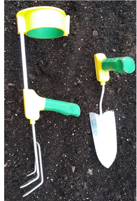
Easy grip arm support cuff, attached to gardening fork (Left). Easy grip trowel, (Right). Source: UT Gardens
