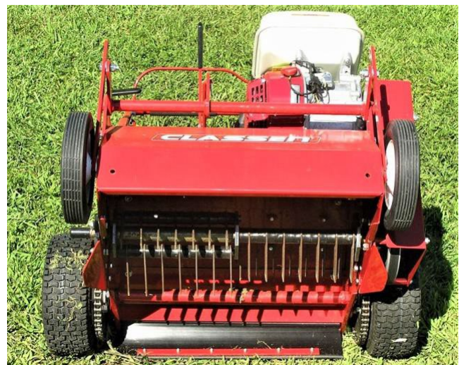
Walk-behind mechanical dethatchers are engineered to slice into the lawn and lift thatch.
