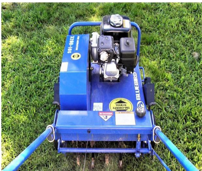
Walk-behind, rotary-motion core aerifiers fitted with hollow coring tines selectively cultivate the lawn by removing soil and plant cores and depositing them on the lawn surface.
