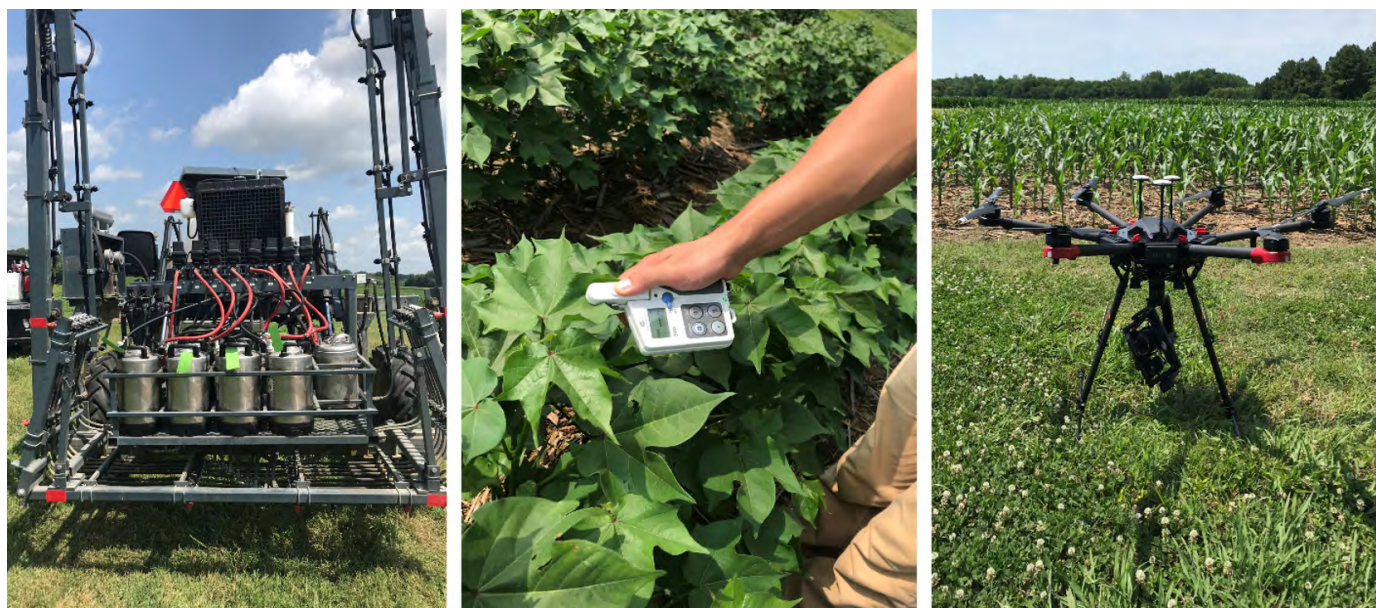
Figure 3. PGR treatments were applied with a Lee Spider (left), then canopy color measurements were made throughout the remaining growing season using a handheld SPAD meter (middle) and UAV imagery (right).
