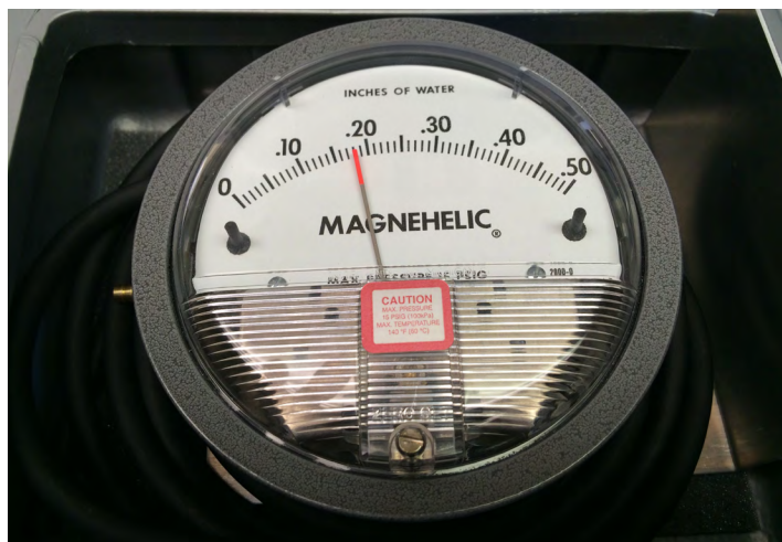
Figure 5. A magnehelic gauge can measure static pressure inside poultry houses. Source: Tom Tabler
