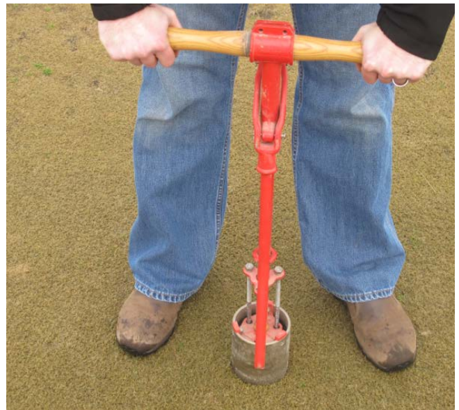
Picture 1. Use a golf course cup cutter to remove samples from areas of concern.
