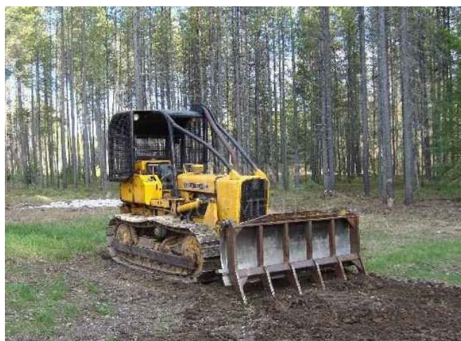
A small dozer with a toothed blade or a small farm tractor with a disc can scarify the ground to improve acorn-ground contact after a bumper acorn crop. Photo Credit: Wayne K. Clatterbuck
