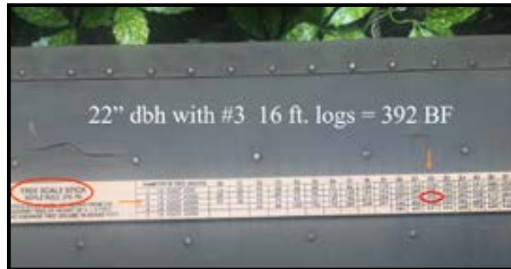
Fig. 6. A standing tree measuring 22" DBH with three 16' logs has 392 board feet using Doyle Scale and FC 78. Source: D. Mercker
