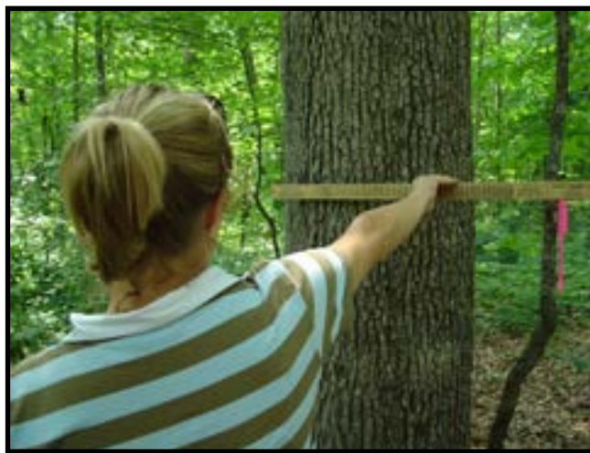
Fig. 1. Measuring DBH using a Biltmore Stick. Source: D. Mercker
