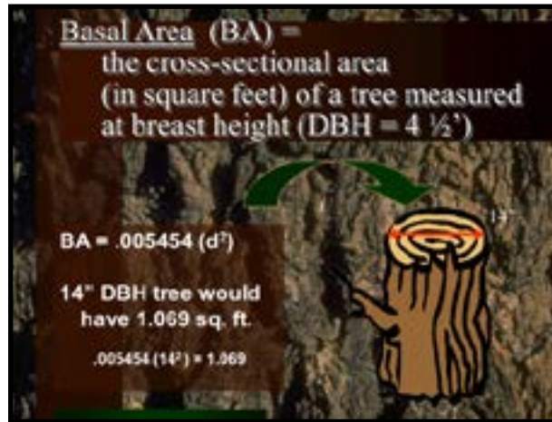
Fig. 2. An example of calculating BA for a 14-inch tree. Source: D. Mercker
